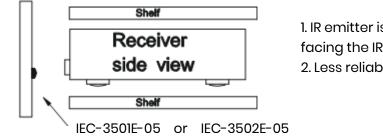
IR emitter is attached to rack door,round shape side facing the IR window
